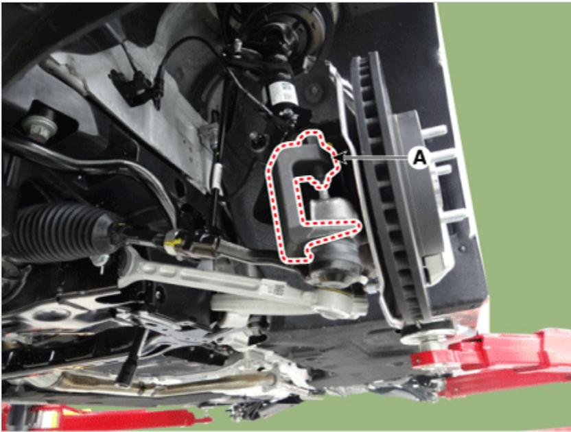
14. Loosen the wheel speed sensor bracket bolt and then remove the wheel speed sensor bracket.
