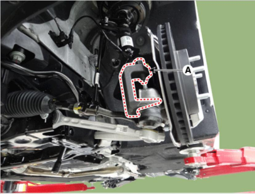
10. Remove the brake hose bracket (A).
