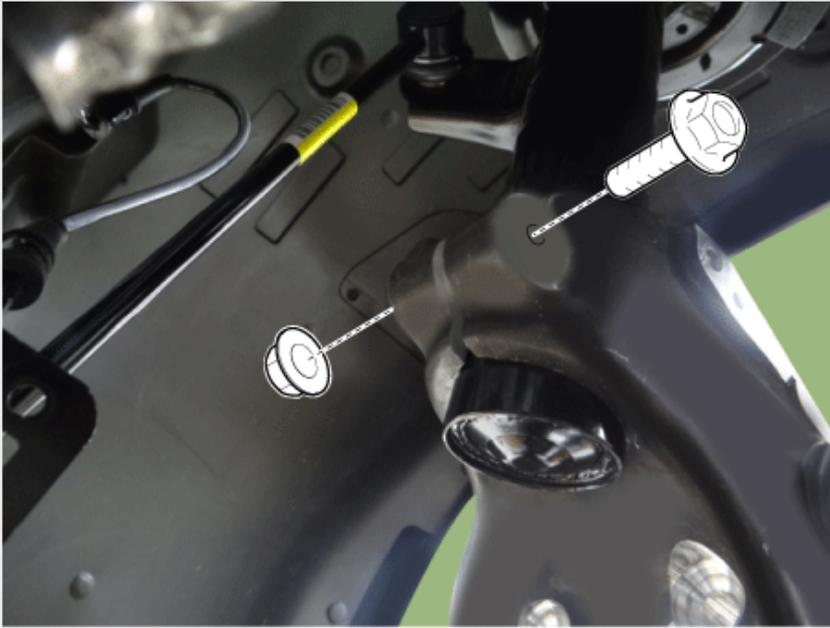
17. Remove the knuckle by using the SST (0K517-J5100).
