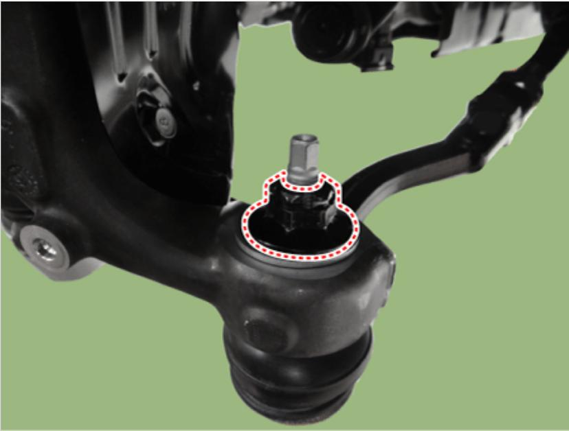
9. Remove the knuckle by using the ball joint remover (A).
