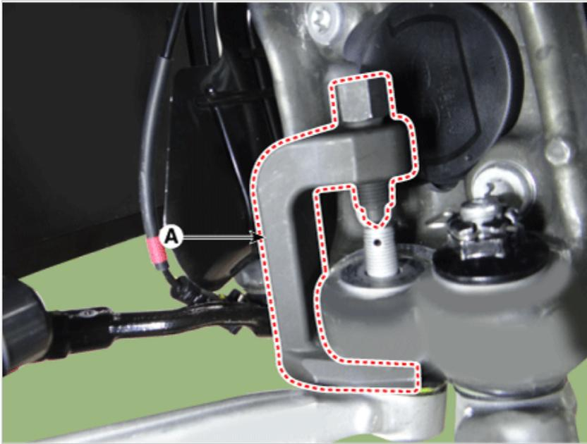
10. Remove the compression arm by using the ball joint remover (A).
