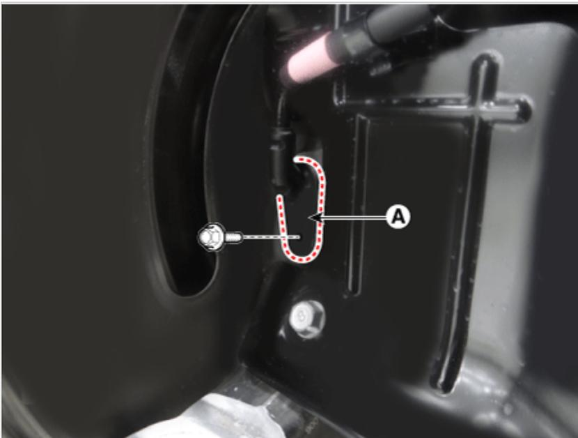
14. Remove the brake cooling cover (A).
