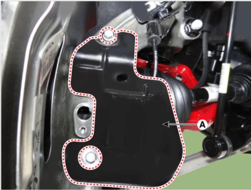
15. Remove the wheel speed sensor bracket (A).
