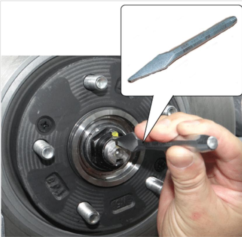
12. Loosen the caulking nut (A) and then separate the hub assembly from the drive shaft.
