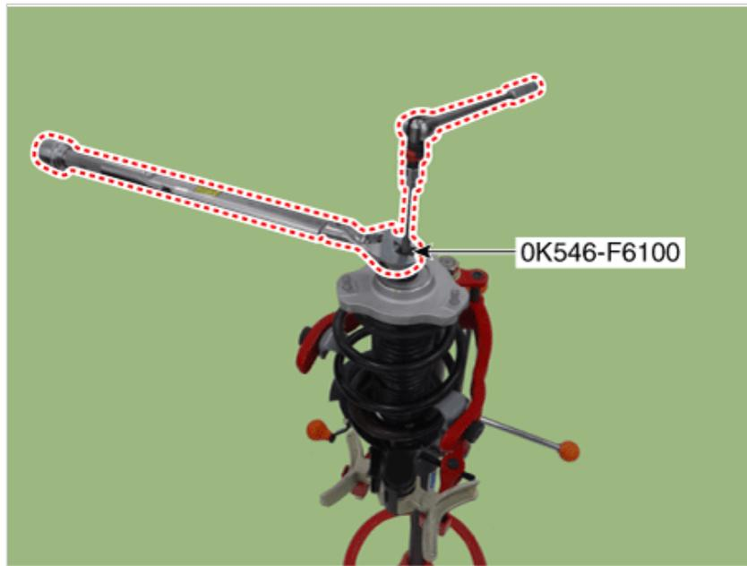
4. Gradually turn the bolt on the spring compressor to slowly release the tension from the spring. Then, disconnect the components.
