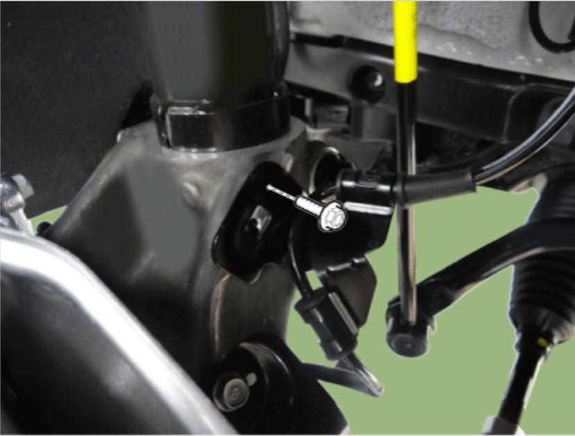
15. Loosen the brake caliper hose bracket bolt.
