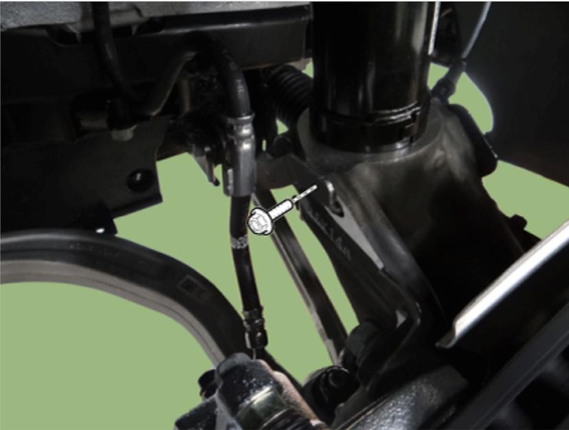
16. Loosen the knuckle upper bolt & nut.
