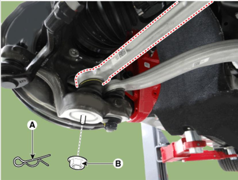
5. Remove the lateral arm by using the ball joint remover (A).
