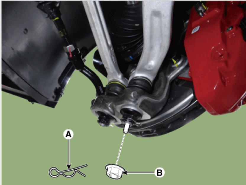
7. Remove the compression arm by using the ball joint remover (A).
